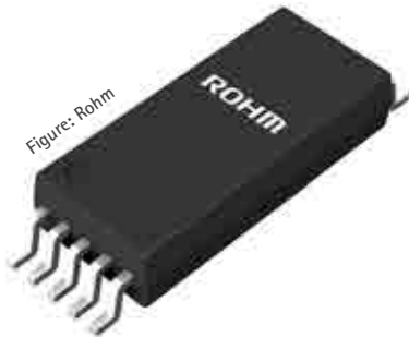
Figure 3: A ROHM SiC-MOS driver with galvanic isolation
