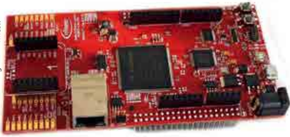
Figure 1: The TC375 lite kit from Infineon can be used with a wide range of development tools for motor controls and safety applications.
