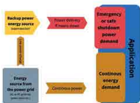
Figure 3: If the energy source fails (e.g. the power network), supercaps can act as backup storage to provide the required energy, e.g. to safely shut down servers.
