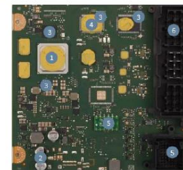
Figure 96: ICAS1 ADAS computer, supplied by Continental
