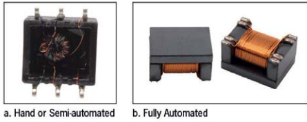
Figure 2: Transformers wound semi-automatically (a) and fully automatically (b).
