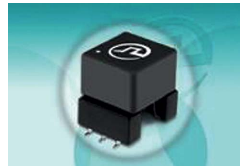
Figure 5: Push-pull transformer with reinforced insulation for separate power supply drivers, 8 mm creepage distance, 5 kV rms insulation (1,000 V rms continuous).
