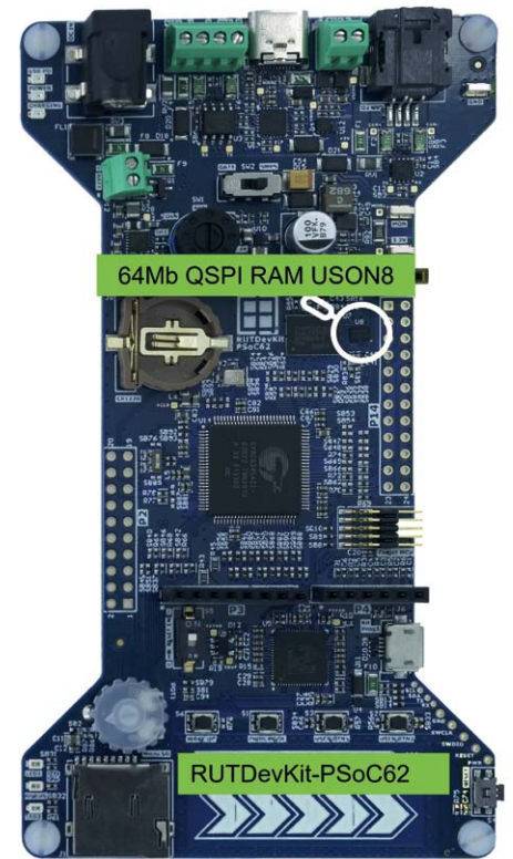
Figure 5: Using external IoT RAM, RDK2 is a modern and easy-to-use hardware platform, especially for the development of wearables and sensors.
