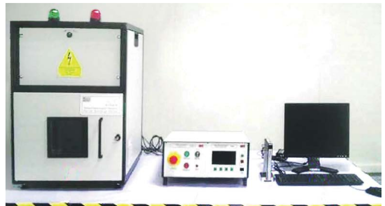
Figure 1: Test equipment for partial discharge testing with test chamber, partial discharge tester, and computer with measurement software.
