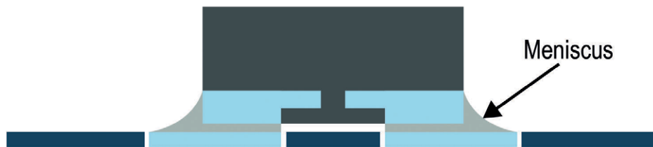
Figure 3: Sketch of the solder meniscus. This can be inspected with an optical camera system to assess the solder result.
