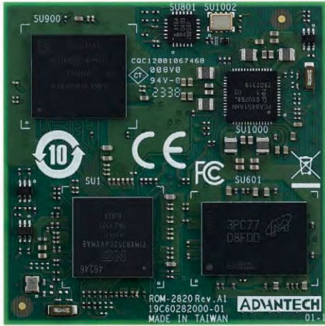
Figure 8: Advantech's ROM-2820 is a powerful SoC (OSM size L) with Edge ML capabilities
