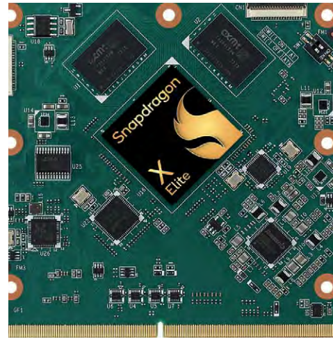
Figure 9: Advantech's AOM-7721 is powered by a Qualcomm X Elite SoC for machine image processing and AI applications
