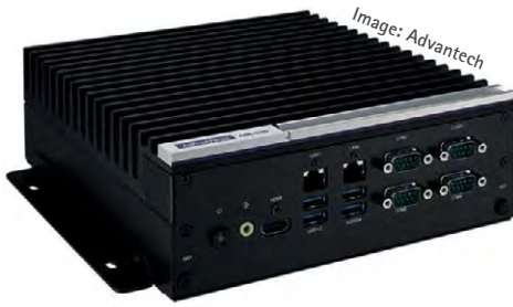
Figure 5: Advantech's AIR-030 AI inference system based on NVIDIA Jetson AGX Orin
